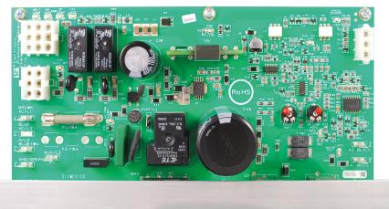
Powerful, quiet, efficient PWM belt speed control, incline control, and console power. Simple direct control inputs and feedback allow your console full control of all basic treadmill functions.
