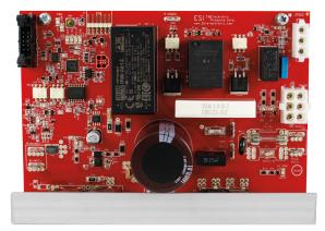
Powerful, quiet, efficient PWM belt speed control, incline control, and console power. Facilitates console requirements with adaptable control inputs and communication protocols. Built-in CPU runs all control loops internally instead of from console, resulting in better control of the motors and ability to add new features. Smart power control, safety, and service monitoring is built in.
